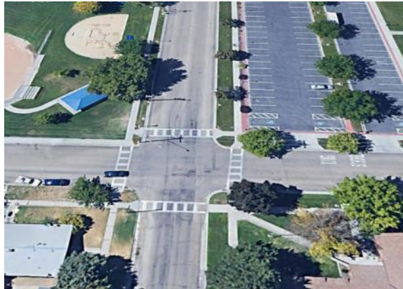
(Above) Adding a two-way stop to force drivers to stop at the gateway entrance to the school gives additional protections to students and park users outside of school activities.
